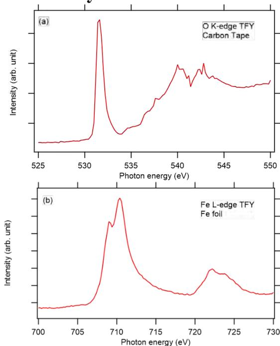
Fig. 1. XAS spectra of (a) O K-edge spectrum of carbon tape and (b) Fe L-edge spectrum of Fe foil measured by PD.
