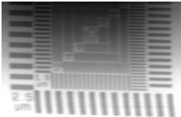
Fig. 3. Resulting image obtained by scanning transmission X-ray microscopy.
