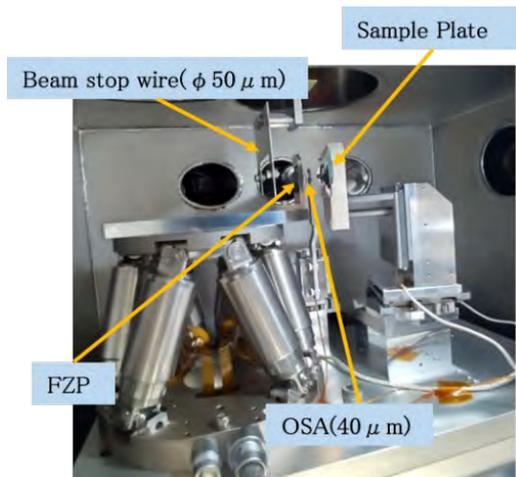
Fig. 2. Photograph of the focusing system.
